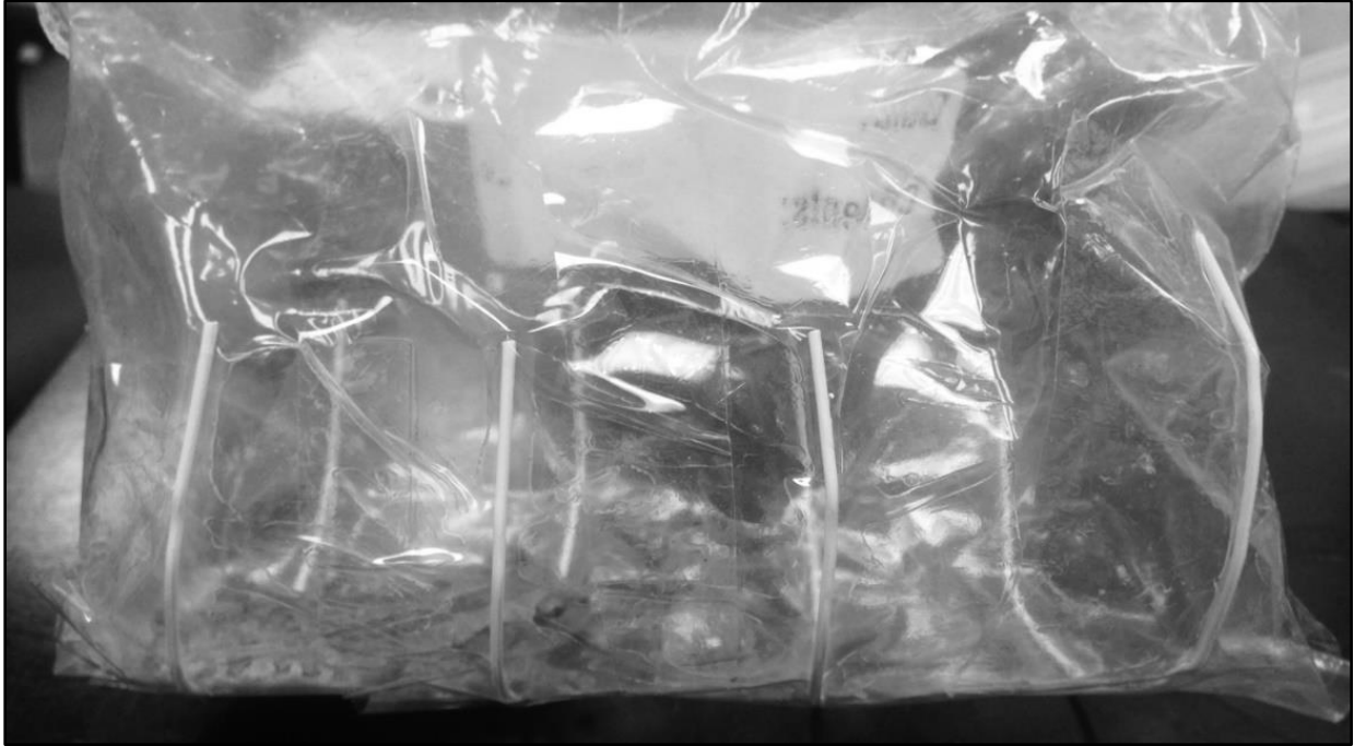
Figure C4. Feeding containment apparatus with one adult Osteopilus septentrionalis for size comparison. Constructed of quart-size zip-top bags with plastic coated paper clips adhered to the outside for structure. Figure and caption adapted from Sauer et al. (2016).
